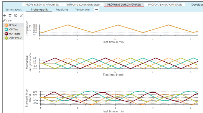
Chronological sequences of temperature, mechanical strain and standard force - IP (orange), OP (blue), CD (red), CCD (green)
